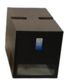
The DBL Series Vacuum pump Noise enclosure consist of two main parts, a base with a door including a frontal window and a top cover place. The installation is very easy and is achieved without tools. Oil mist filter fits inside or outside of the enclosure. Convenient access for system checks and maintenance by the front and the top.
